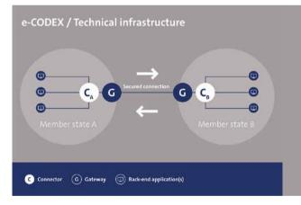
The technical infrastructure consists of a connector and a gateway. The installation of the gateway ensures a secured connection with a gateway in another Member State. The connector carries out the adaptations required for receiving encrypted data by the corresponding service provider in another Member State
